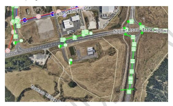
Servicing: Green: Stormwater, Red- Wastewater, Blue- Water
