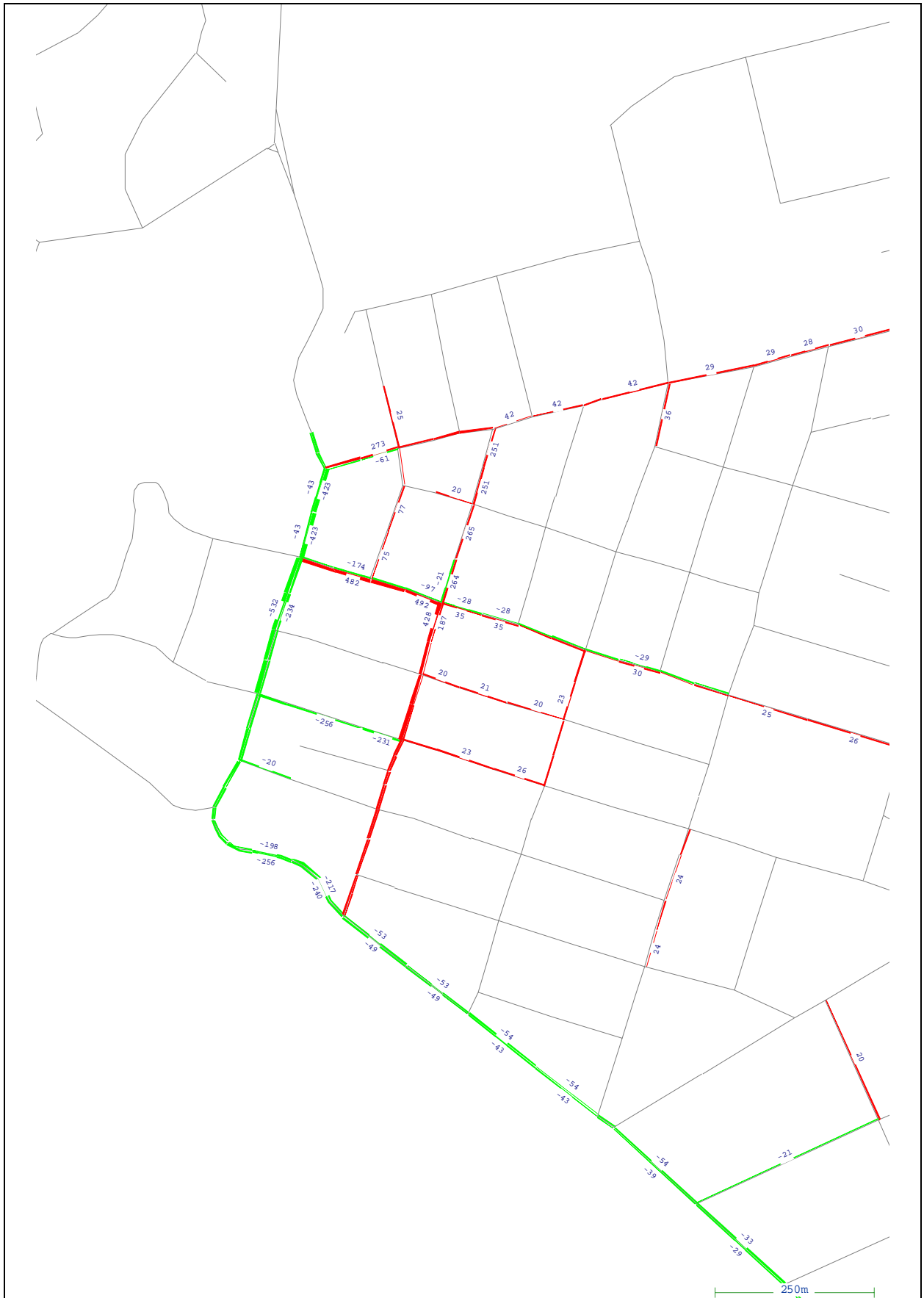
Taupo Town Centre Modelling 2021 PM Peak Traffic Volumes Change Plot Base v Stage 1 Figure 16 Gabites Porter
