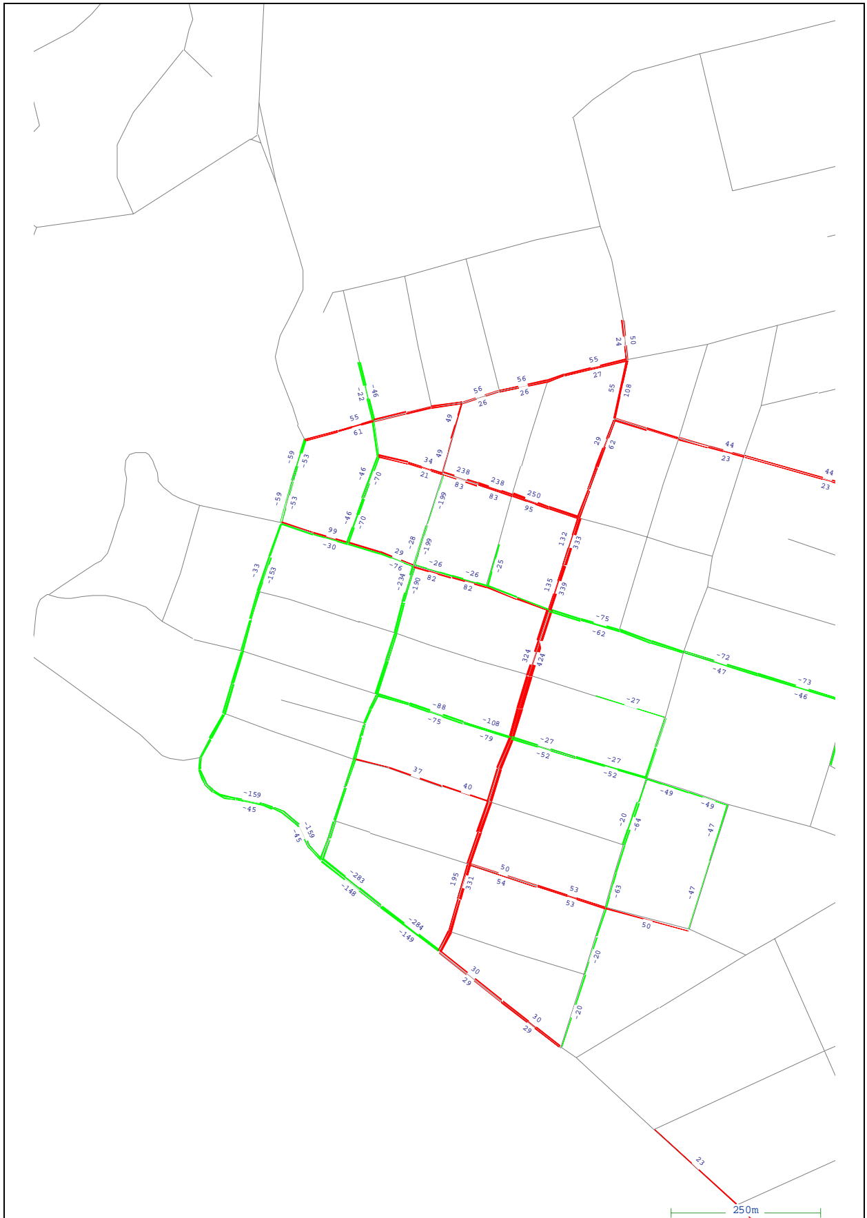
Taupo Town Centre Modelling 2011 PM Peak Traffic Volumes Change Plot Stage 1 v Stage 2 Figure 26 Gabites Porter
