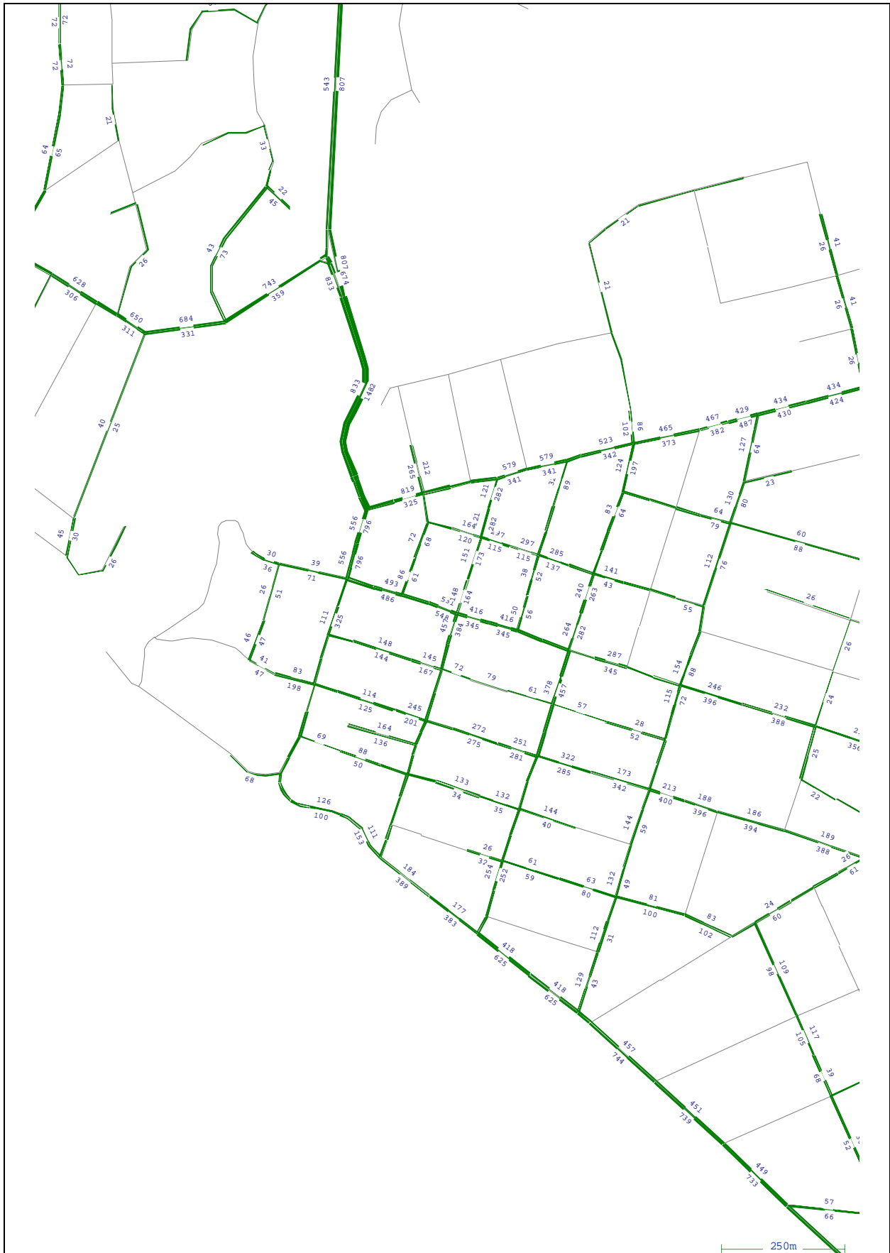
Taupo Town Centre Modelling Stage 2 2011 AM Peak Traffic Volumes Figure 21 Gabites Porter
