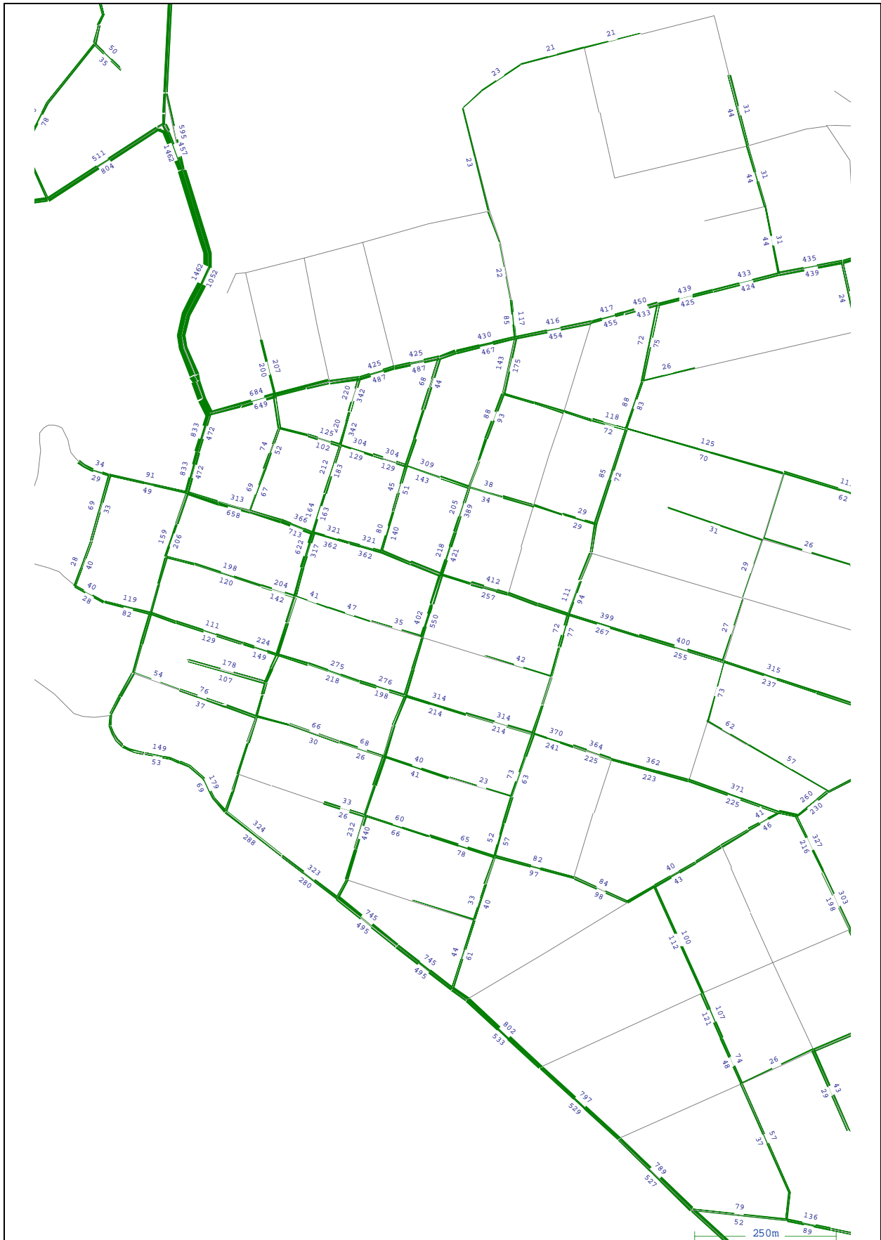
Taupo Town Centre Modelling Stage 2 2011 PM Peak Traffic Volumes Figure 22 Gabites Porter
