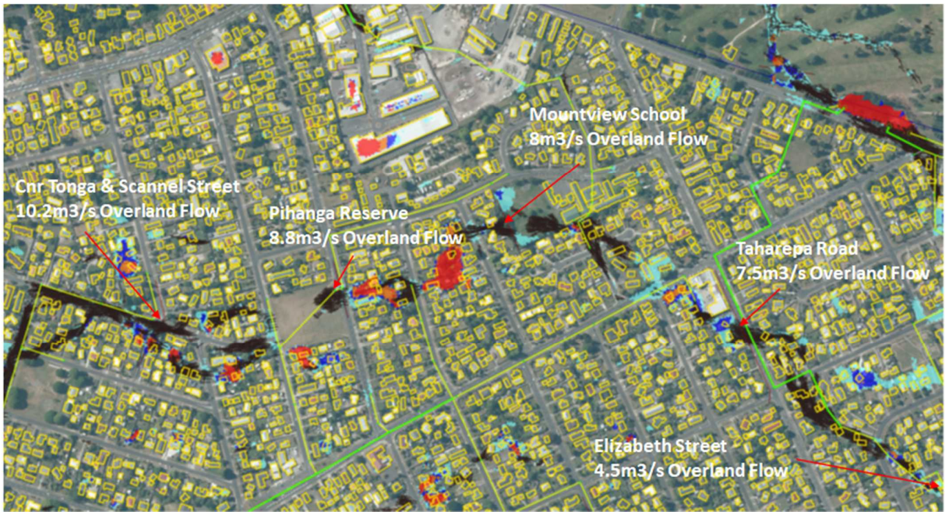
Figure 1. 100-Year Overland Flows Quantified within the Elizabeth Street Gully System.
