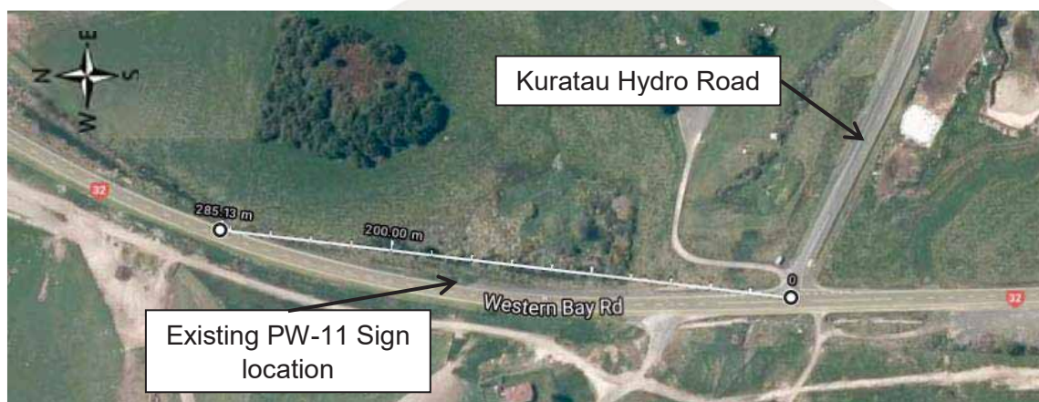
Figure 2: Visibility north of Kuratau Hydro Road limited by horizontal curve
