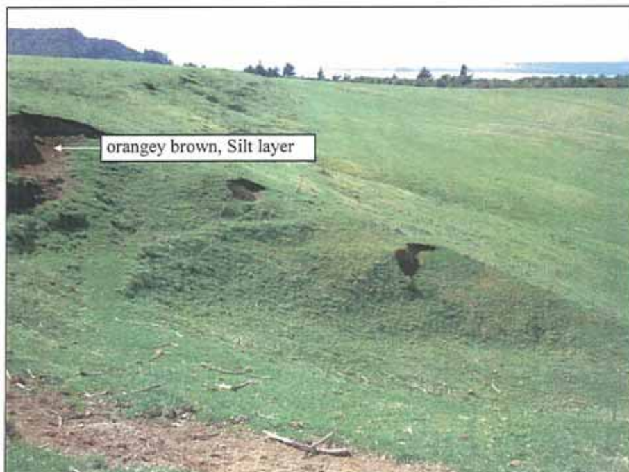
Fig. 3: Minor slumps along the east-west oriented slope that separates the upper terrace from the low area. Lake Taupo can be seen in the distance to the east.
