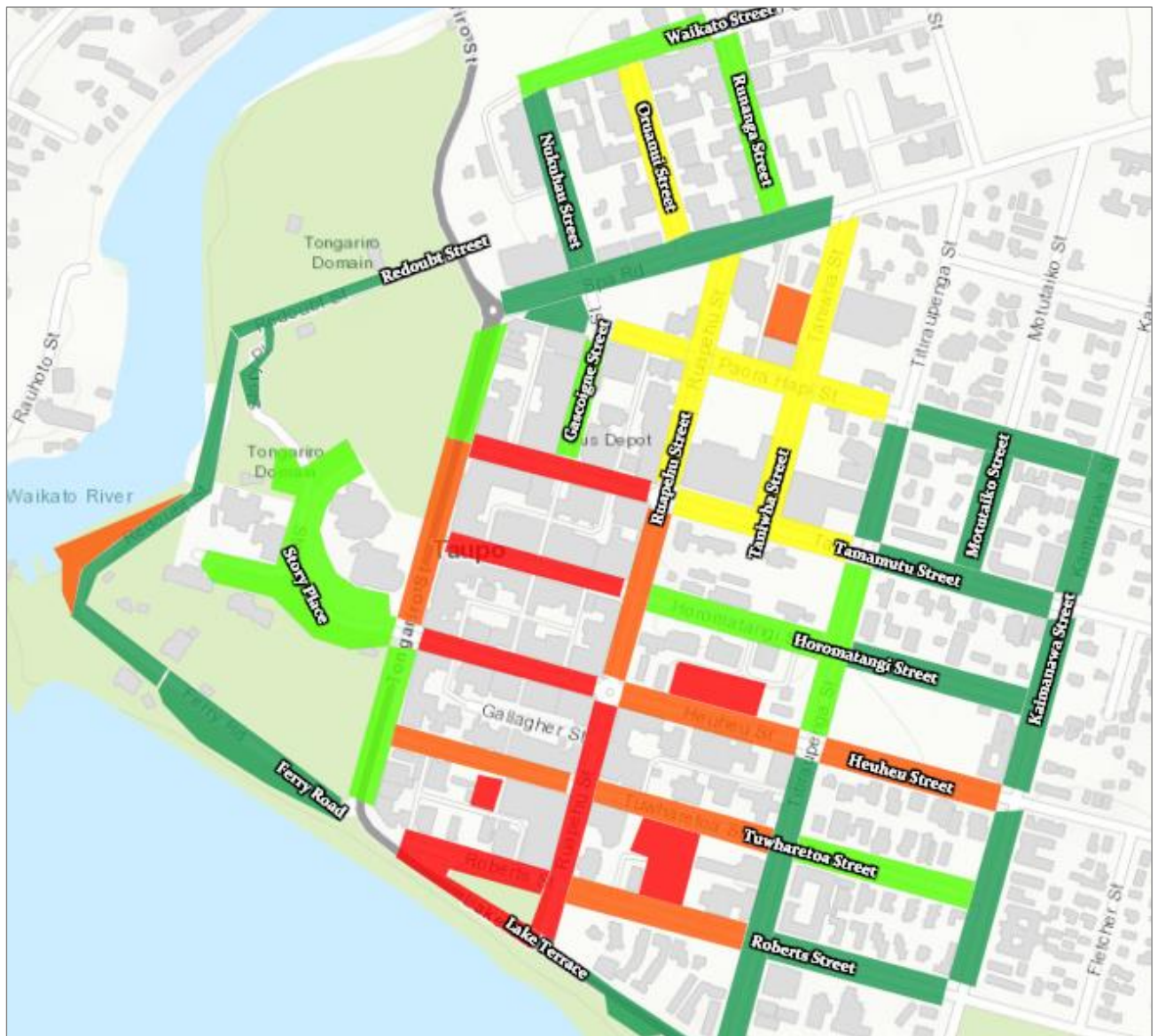
Figure 1.2 Parking survey occupancy rates
