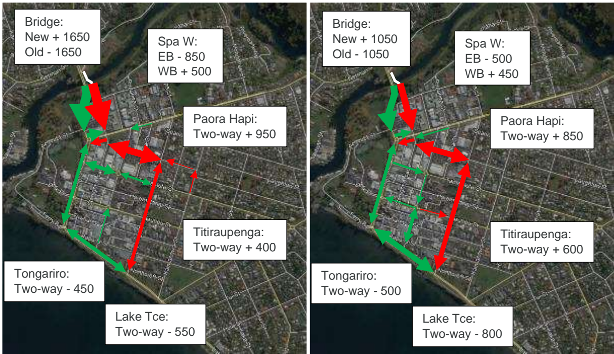
Figure 4.17 Option 1 with Traffic Calming Change in Volume Morning Peak (Left) and Evening Peak (Right)
