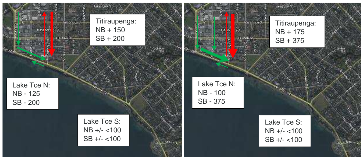
Figure 4.12 Option 1 Change in Volume Morning Peak (Left) and Evening Peak (Right) - Lake Tce View
