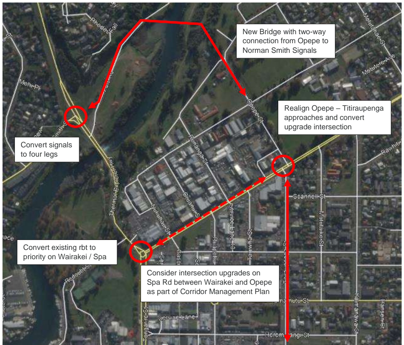
Figure 4.6 Infrastructure Changes for Eastern Bridge Connection via Opepe Street
