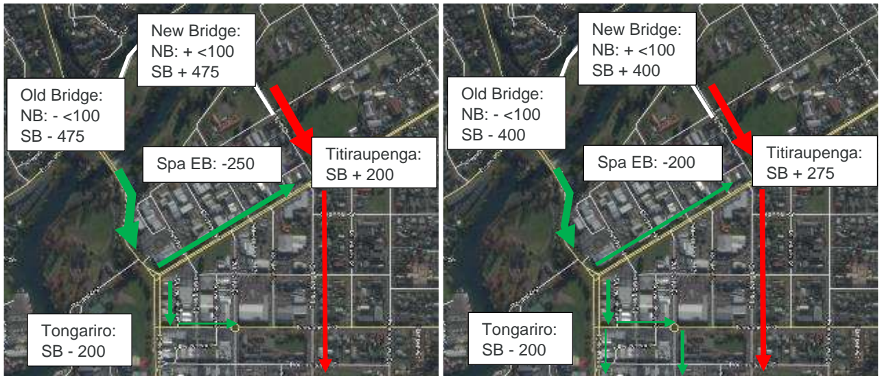
Figure 4.10 Option 2 Change in Volume Morning Peak (Left) and Evening Peak (Right) - Spa Road View
