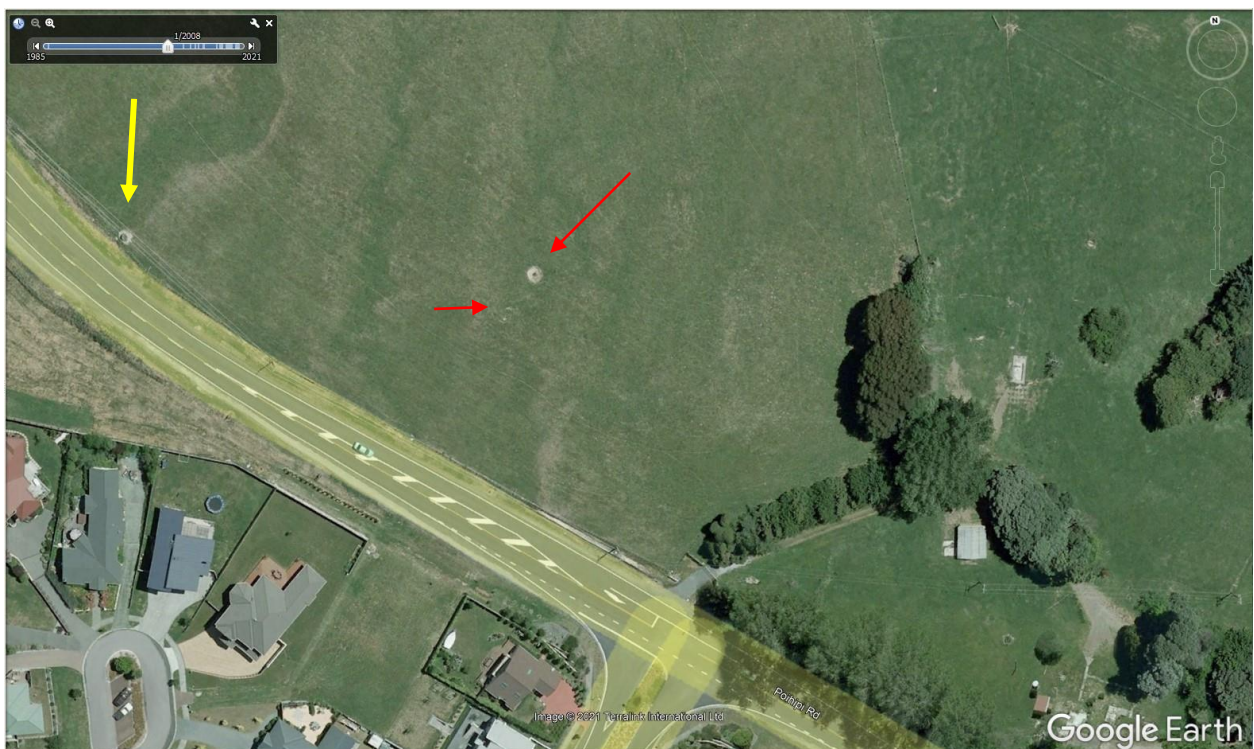
Figure 3: Depressions in Area C indicated by red arrows (2008). Stock water trough yellow arrow.
