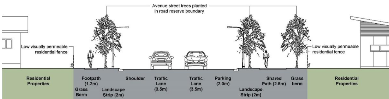
Figure 7-5: Cross section illustrating the roading design
