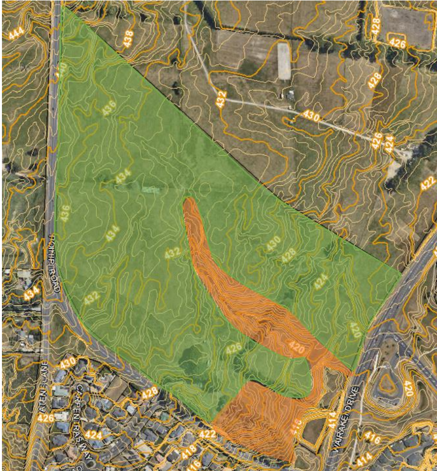
Figure 20: Indicative estimated cut and fill depth areas at Site 3 (green = estimated 1-2m, orange 2m+)
