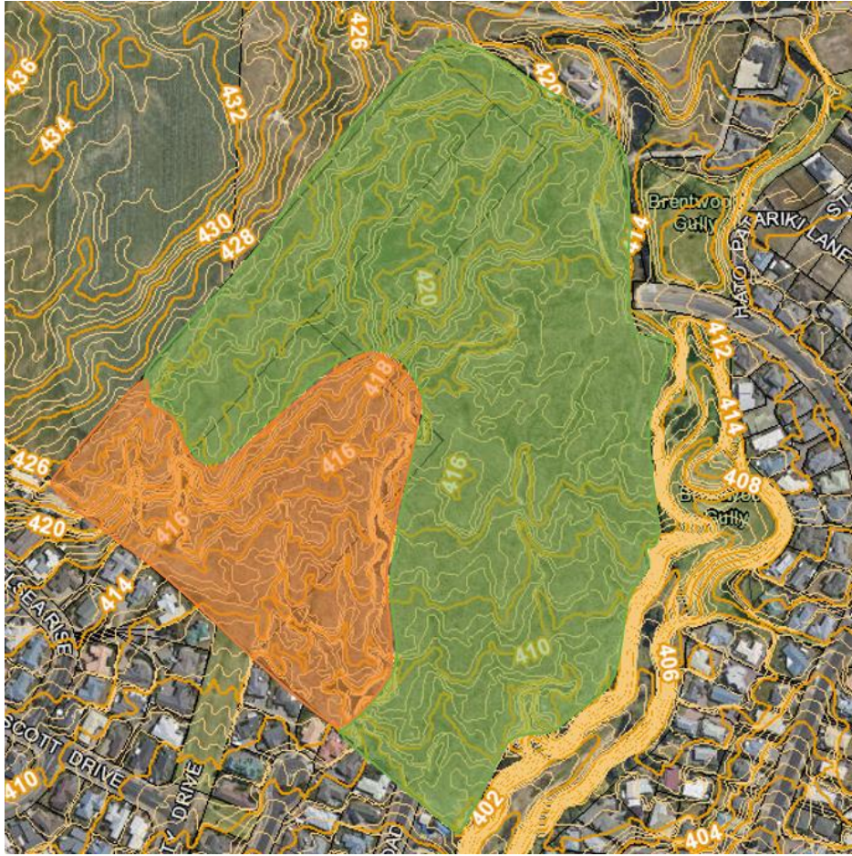
Figure 22: Indicative estimated cut and fill depth areas at Site 6 (green = estimated 1-2m, orange 2m+)
