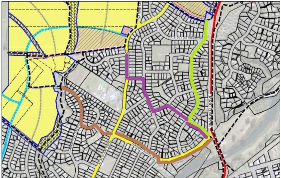
Figure 5: Indicative active mode routes from the Site to the Wairakei Drive / Tongariro Street / Norman Smith Street intersection. Green route is from Poihipi Road, purple route is from Herapeka Street, and brown route is from Lakewood Drive (refer to Appendix A for the original diagram)
